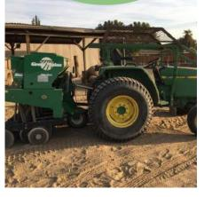
No-till drills, which will maximize germination, are the most precise and expensive seeding method for cover crops.
